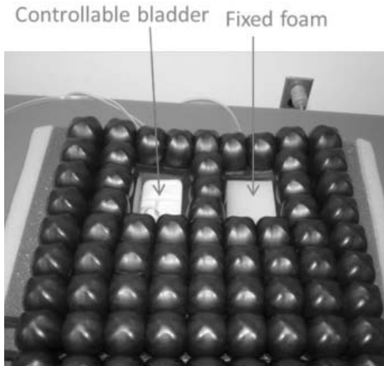
Figure 1. Custom cushion for testing blood flow response to loading.
