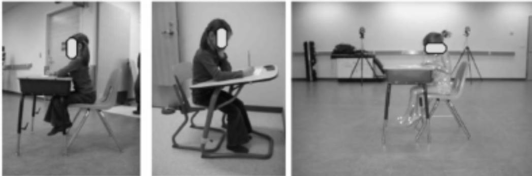
**Figure 1:** a) Child seated at the standard school chair and adjustable height desk; b) Child seated at the ergonomic table and chair adjusted to the manufacturers specifications; c) Reflective spheres positioned on anatomical landmarks located on the head, shoulders, pelvis, legs and feet.
